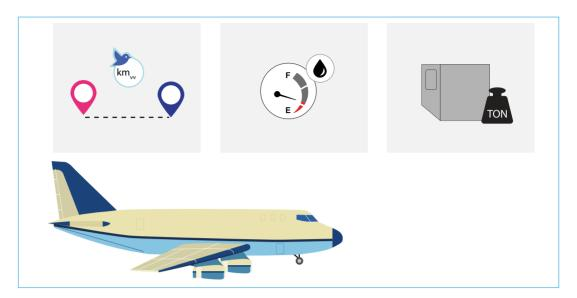
In principle, allocating  $CO_{2e}$  emissions to cargo is relatively simple in the case of a cargo aircraft: the great circle distance between the airport of departure and airport of destination is known, as are the aircraft's consumption and the weight of each component of the cargo.
